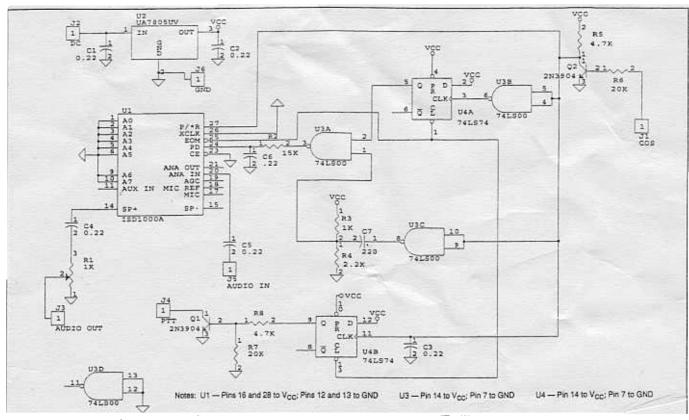
Figure 1. Schematic Diagram for the Simple Simplex Repeater.
